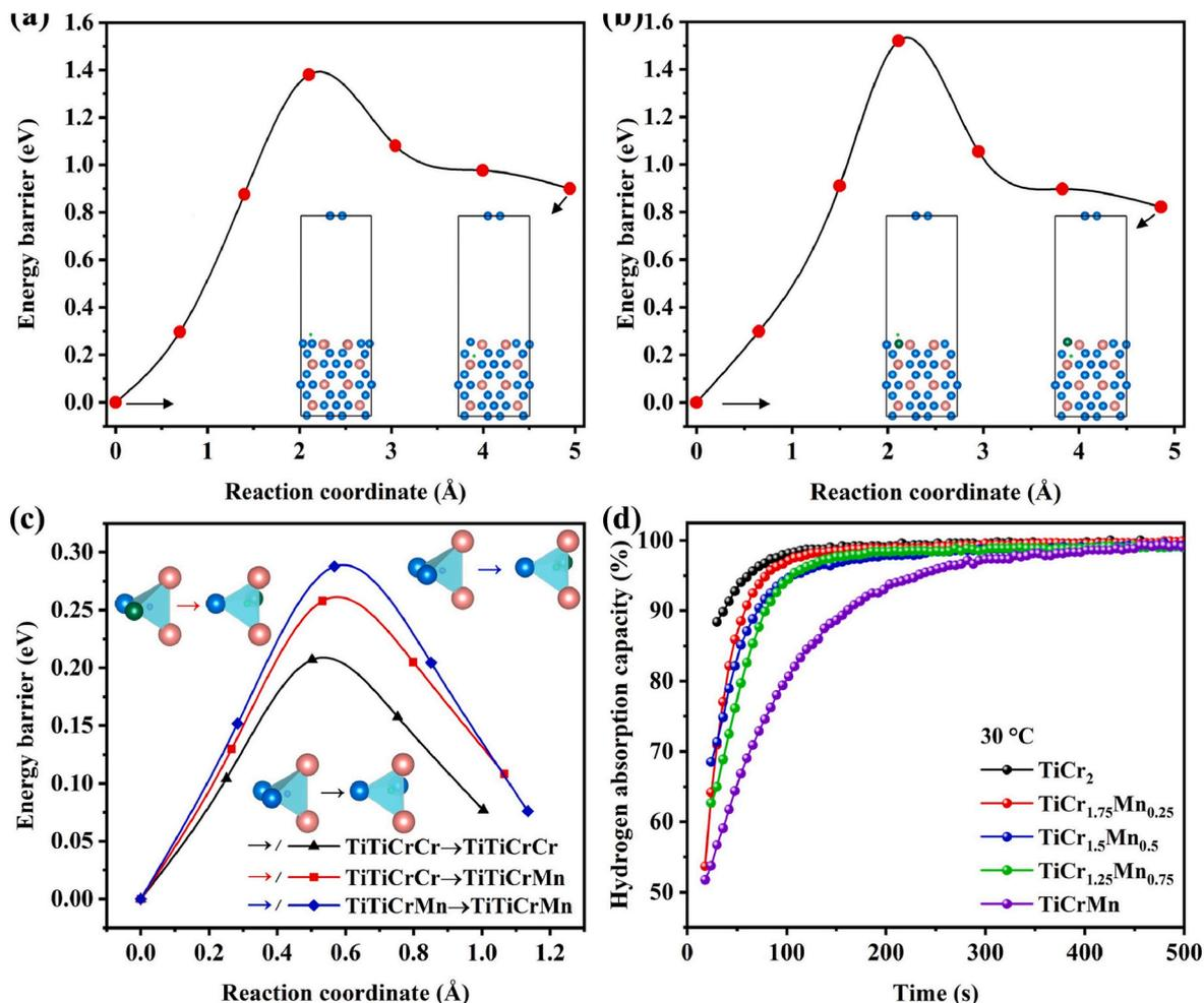
**Fig. 8.** Calculated diffusion energy barriers of an H atom from surface to TiCr<sub>2</sub> bulk (a) and TiCr<sub>2-x</sub>Mn<sub>x</sub> bulk (b), H atom diffuses from 6h<sub>1</sub>-6h<sub>2</sub> tetrahedral interstices (c) and the normalized isothermal hydrogen absorption curves of TiCr<sub>2-x</sub>Mn<sub>x</sub> alloys (d).
