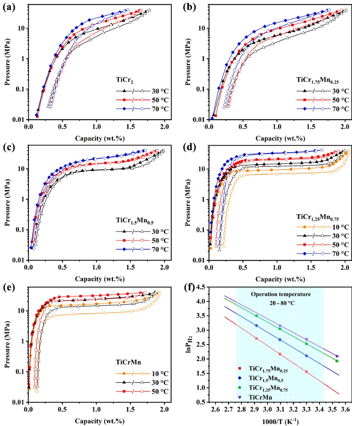
Fig. 5. Hydrogen absorption/desorption performance of  $\text{TiCr}_{2-x}\text{Mn}_x$  alloys at 10, 30, 50 and 70 °C (a–e) and Van't Hoff plot (f).
