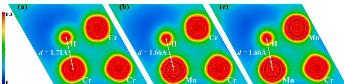
Fig. 3. Charge densities of  $\text{A}_2\text{B}_2$  tetrahedral interstices of  $\text{TiCr}_{2-x}\text{Mn}_x\text{-H}$  alloys: Ti–Ti–Cr–Cr interstice (a), Ti–Ti–Cr–Mn interstice (b), Ti–Ti–Mn–Mn interstice (c).
