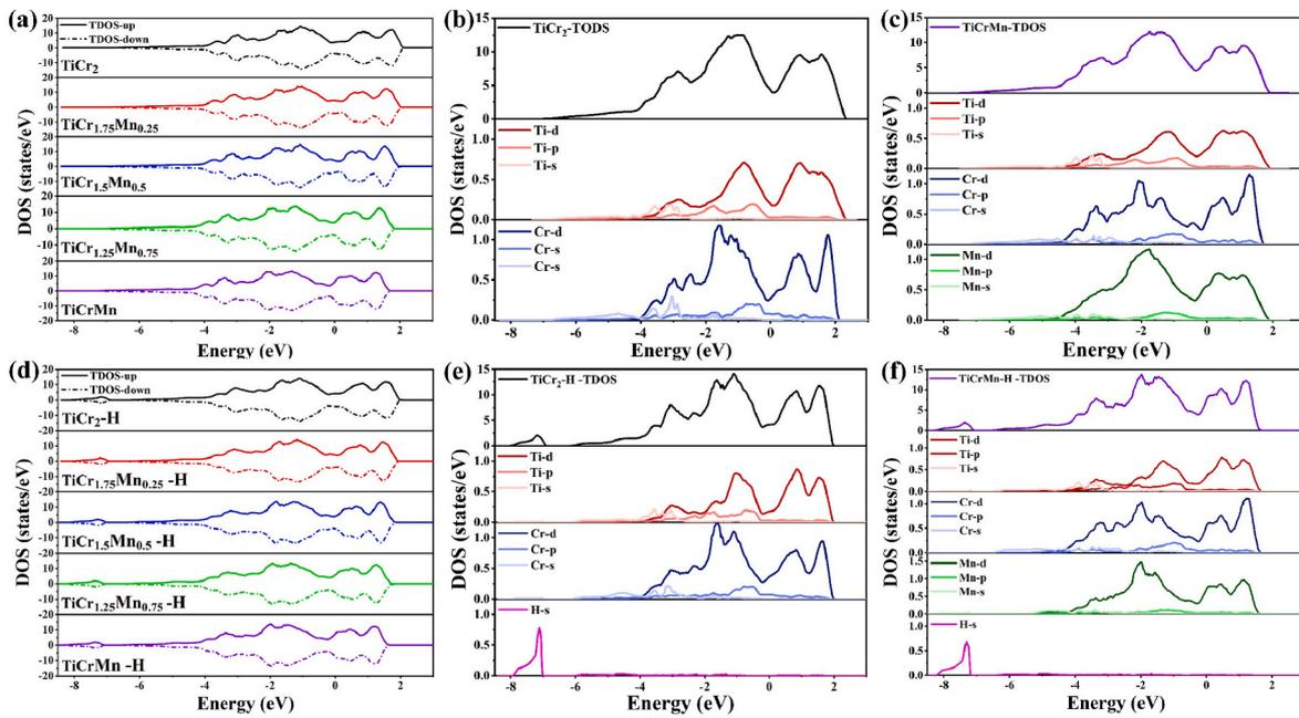
Fig. 2. Total and partial DOS of the most stable structure of  $\text{TiCr}_{2-x}\text{Mn}_x$  and  $\text{TiCr}_{2-x}\text{Mn}_x\text{-H}$  system.
