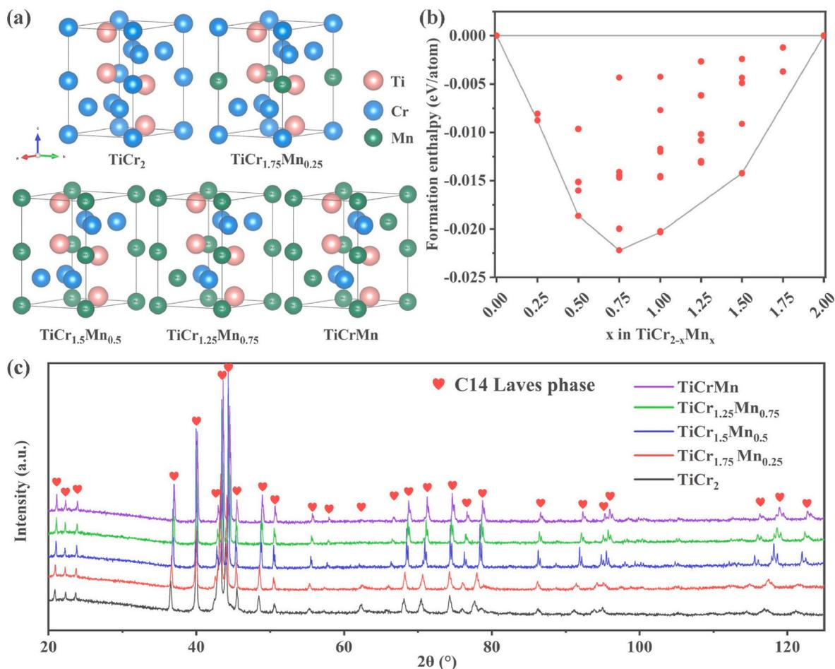
**Fig. 1.** The structure stability of  $\text{TiCr}_{2-x}\text{Mn}_x$  alloys: the site of Mn substituted for Cr in  $\text{TiCr}_{2-x}\text{Mn}_x$  alloy in DFT (a), formation enthalpy (b) and XRD patterns of  $\text{TiCr}_{2-x}\text{Mn}_x$  annealed alloys (c).
