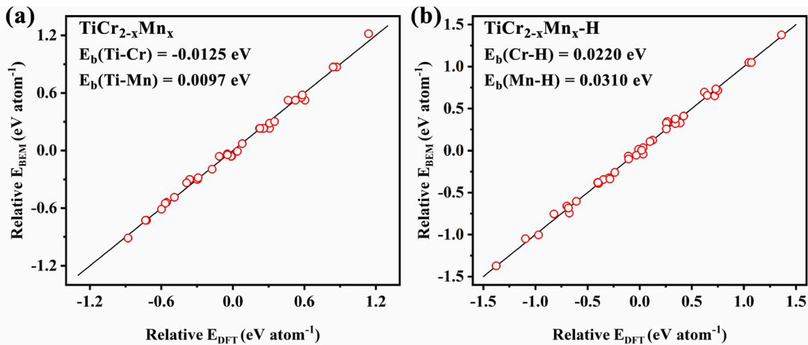
Fig. 4. Total energies of  $\text{TiCr}_{2-x}\text{Mn}_x$  and  $\text{TiCr}_{2-x}\text{Mn}_x\text{-H}$  systems obtained by DFT calculation and by BEM method (red circle).
