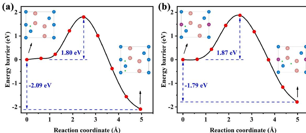
Fig. 7. Dissociation of  $\text{H}_2$  molecules on Ti3–Cr2–Cr3 HS of  $\text{TiCr}_2$  (1 1 0) surface (a) and Ti3–Mn2–Cr3 HS of  $\text{TiCr}_{2-x}\text{Mn}_x$  (1 1 0) surface (b).
